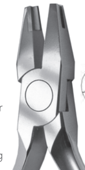
Tweed Arch Bending Plier - .060 Part # GCOA-012 Length: 117mm Maximum Bending Capacity: Rectangular wires up to .022"x.028" Beaks are .060" wide, parallel at .020" opening
