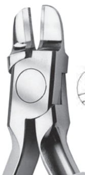
Tweed Arch Bending Plier - .043 Part # GCOA-140 Length: 117mm Maximum Bending Capacity: Rectangular wires up to .022"x.028" Beaks are .043" wide, parallel at .020" opening
